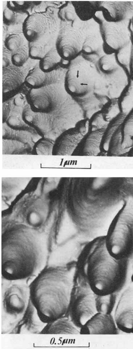
Fig. 7. TEM of surface replica from unprotected top surface of space exposed Specimen I.
